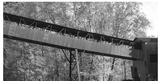
Above is a section of the "button and rope" conveyer system. It carried the coal from top to bottom. It was designed for a gentler transport of coal.
